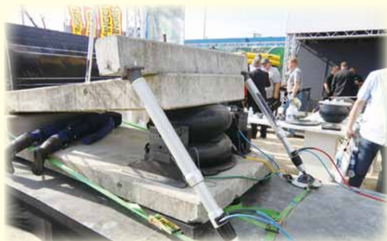
• 氣墊積與氣動式支撐系統 Air lifting bags and pneumatic support system
